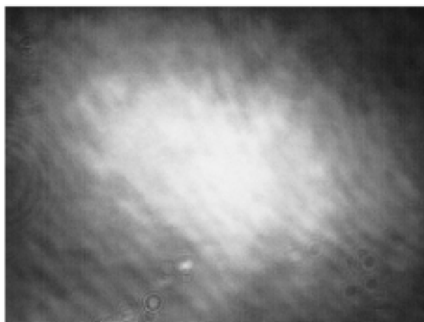
Figure 3. Top: fullerodendrimers with peripheral C 60 units ( 4 ) [12] and containing C 60 spheres at each branching unit ( 5 ). [13] Bottom: Brewster angle microscopy image for 4 at \lambda = 480 \text{ \AA}^2 , the stripes that can be seen are interferences due to the laser light.
